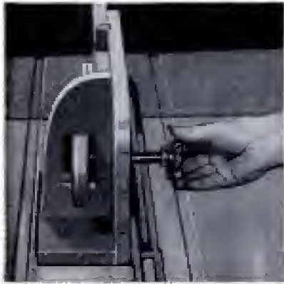
Before running cut on work, right, adjust clamp arm to parallel position with hand wheel as above
